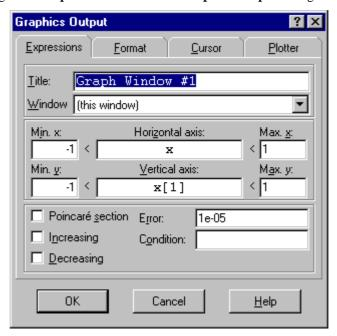
Change the **Min. x**, **Max. x**, **Min. y** and **Max. y** entries and press Enter to select as new window the square -4 < x, dx/dt < 4.
